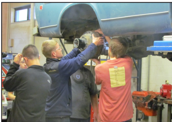
Austin Dedrick assists classmate Ryan Elmore with replacing the brake drum during class. Students routinely volunteer their own cars to practice on for free repairs when the class studies auto repair skills.
